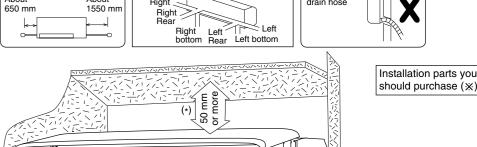
nstallation plate [1 50 mm Sleeve (X) (Gum Type Sealer) Bend the pipe as
